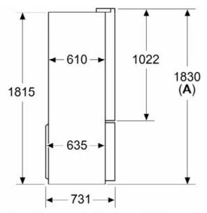
A: Front is adjustable from 1830 to 1847, with front levelling feet fully extended B: Add 25 for fixed spacers on back
