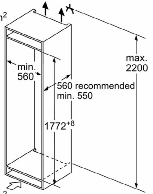
The specified unit door dimensions are valid for a door gap of 4 mm.
