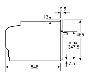
measurements in mm
