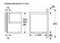
A: Overhang at top: Recess 362: 6 mm Recess 365: 3 mm B: Overhang at bottom: 14 mm
