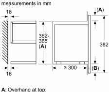
A: Overhang at top: Recess 362: 6 mm Recess 365: 3 mm
