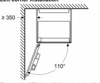
If using the 92° hinge limiter, the min. distance to the wall is only 100 mm  $\,$
