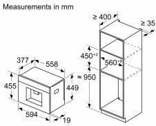
Bean and water containers are removed from Recommended installation height 950–1450 mm
