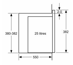
measurements in mm
