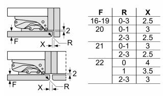
The gap dimensions recommended in the table must be adhered to in order to ensure that appliance doors do not collide with anything when they are opened, and to avoid causing damage to kitchen units. 1/
